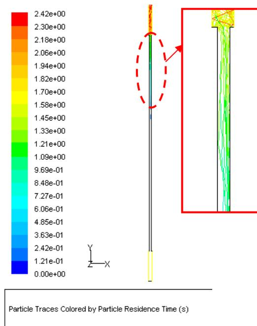
Figure 4. Oxygen bubbles trajectories
