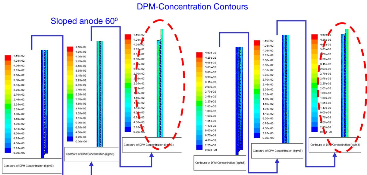
Figure 10. Oxygen bubbles concentration
