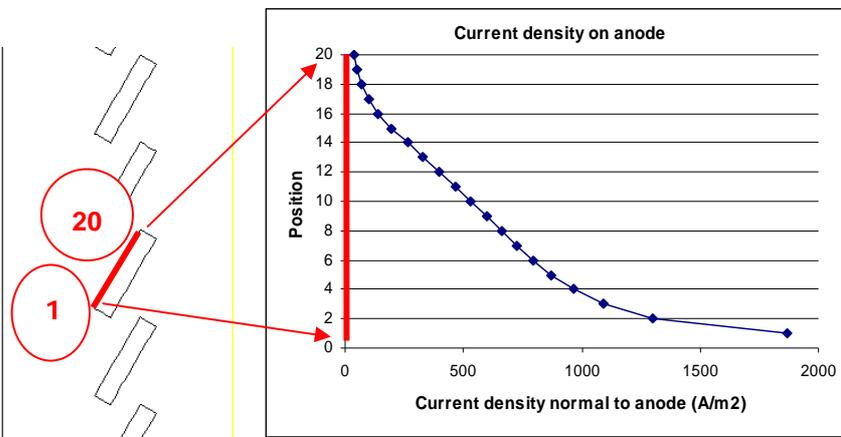
Figure 8. Current density normal to anode for sloped configuration
