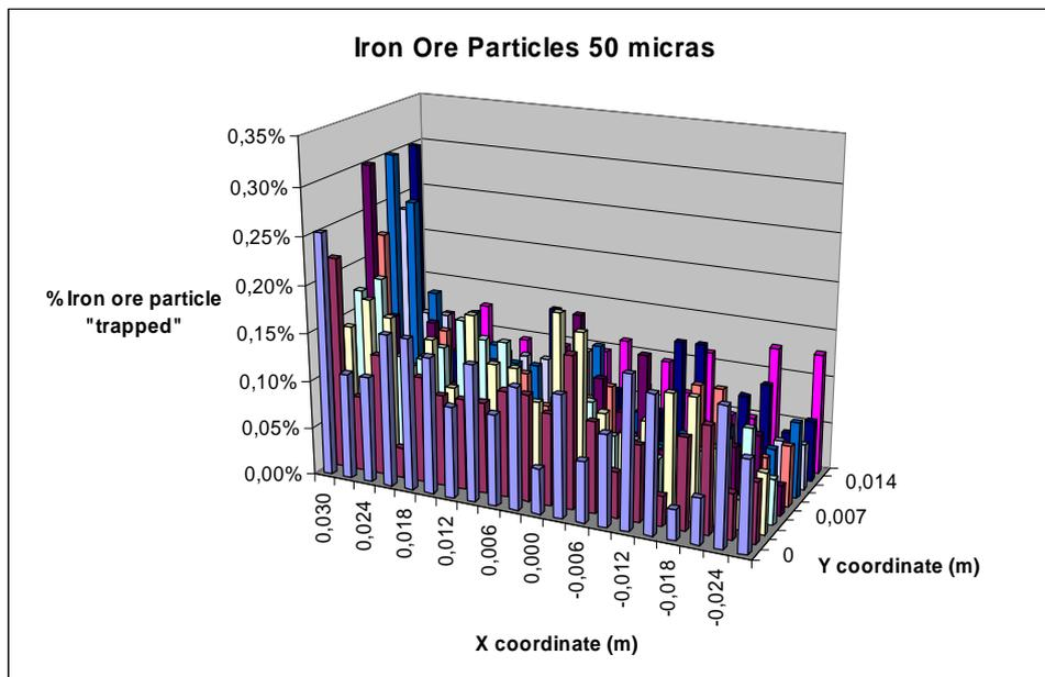
Figure 20. Percentage of particles of 50 µm “trapped” at each cathode subdivision
