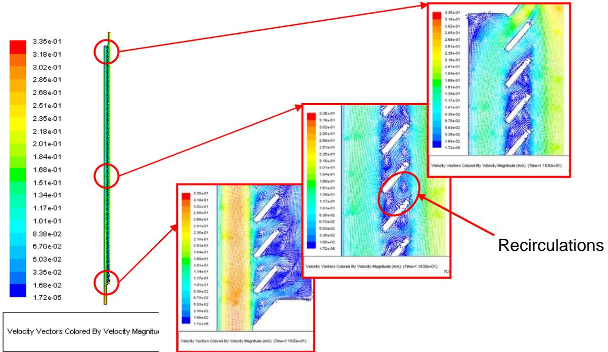
Figure 7. Velocity Vectors for the sloped anode 50° geometry
