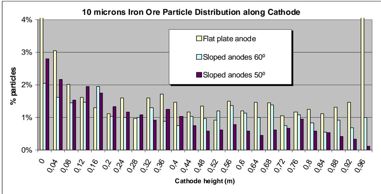
Figure 12. Accessibility of iron ore particles to the cathode
