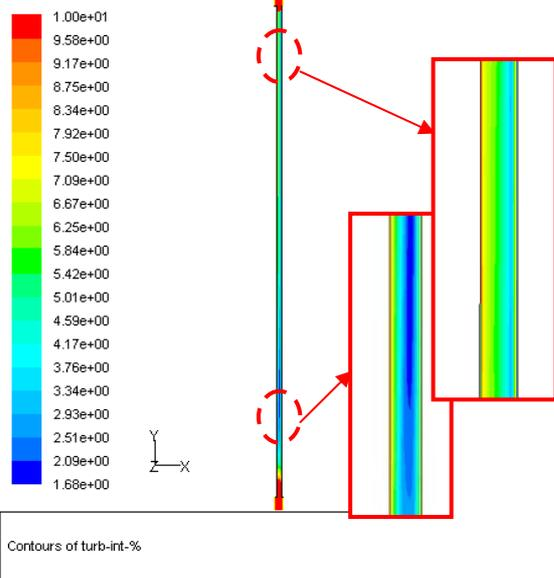
Figure 3. Turbulence intensity for flat plate anode configuration
