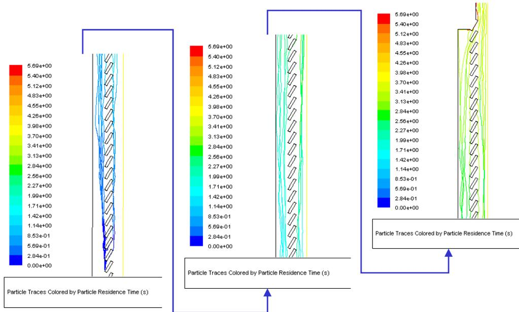
Figure 9. Trajectories of O<sub>2</sub> bubbles generated at the tip of the anode closer to the cathode (sloped anode 60° configuration)
