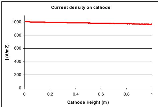
Figure 5. Current density on cathode for flat plate anode configuration
