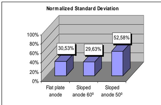
Figure 13. Normalized standard deviation of accessibility of iron ore particles to the cathode
