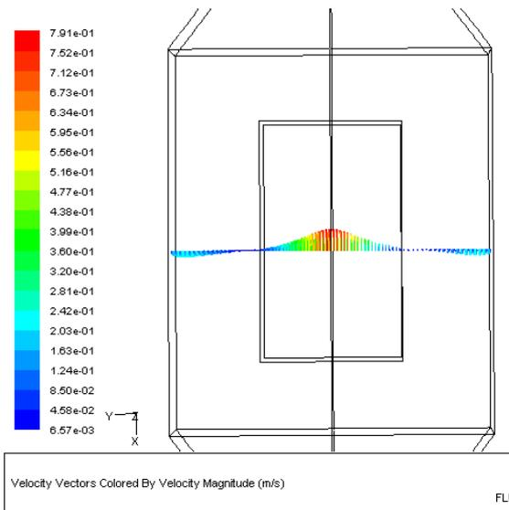
Figure 16. Velocity vectors in a transversal plane (top view)
