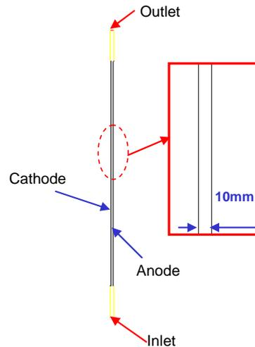
**Figure 1.** Geometry of the flat plate anode (electrode's height 1 m)
