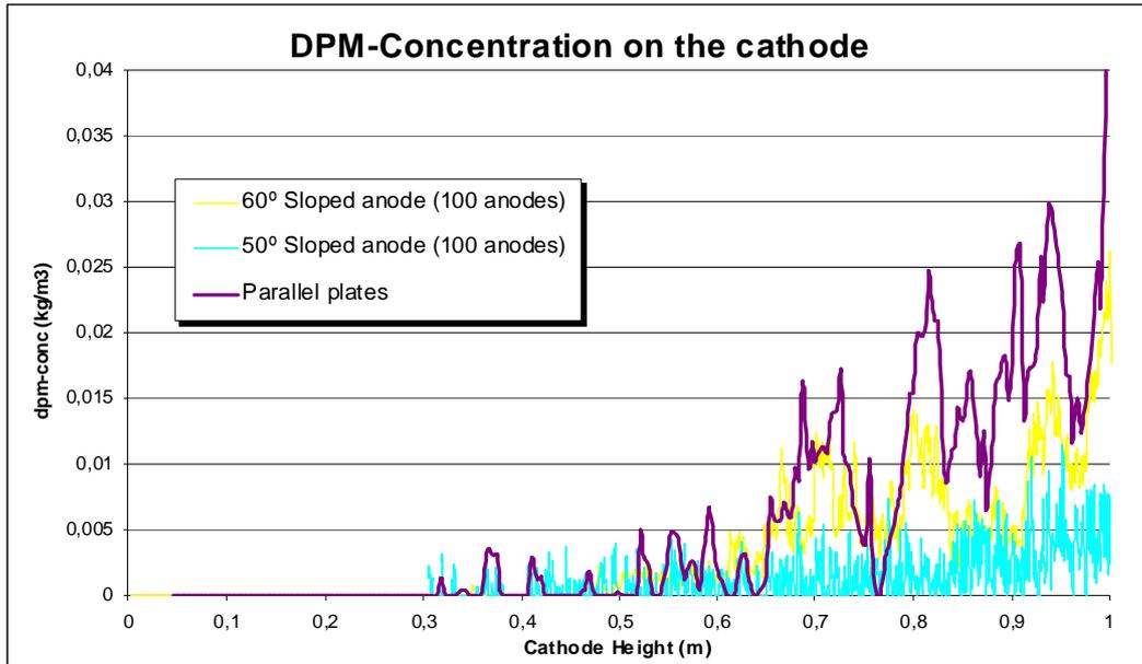
Figure 11. DPM-concentration (O<sub>2</sub>) on cathode
