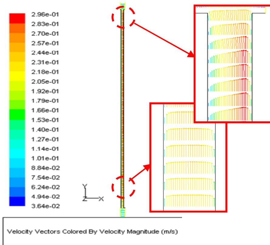
Figure 2. Velocity Vectors for the flat plate anode
