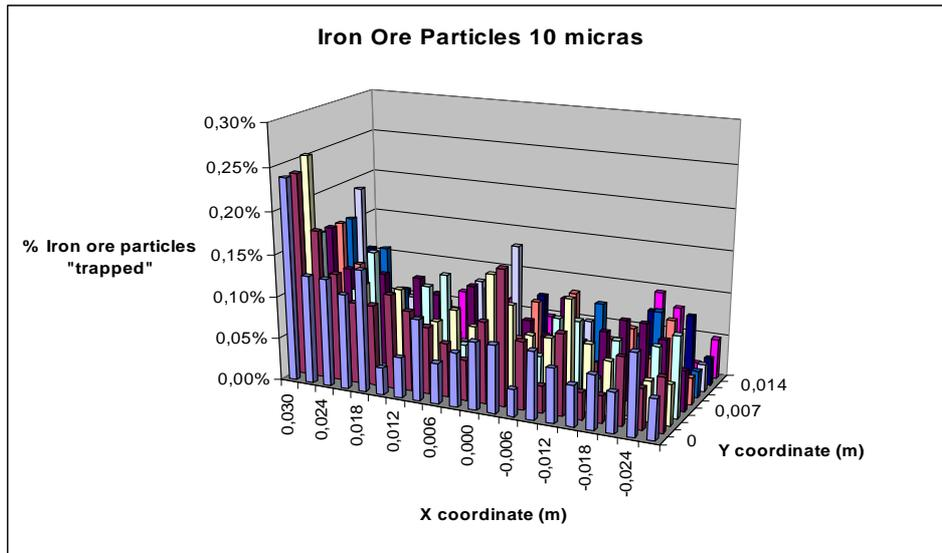
Figure 19. Percentage of particles of 10 µm “trapped” at each cathode subdivision
