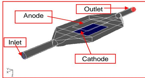
Figure 14. Geometry of the horizontal laboratory cell
