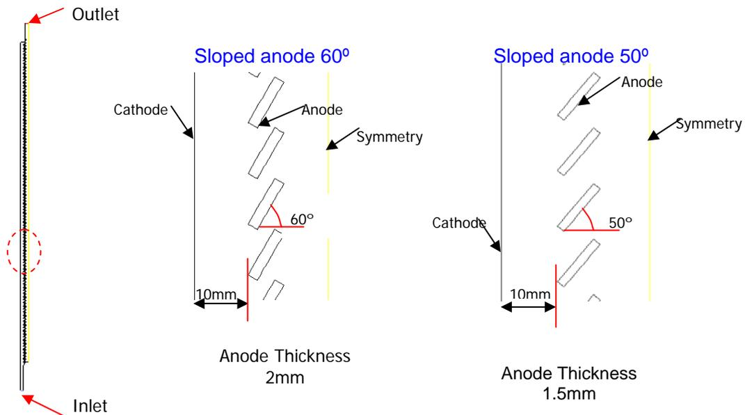
Figure 6. Geometry of the sloped anodes configurations
