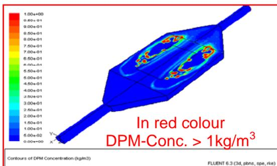
Figure 17. Contours of oxygen bubbles concentration ( $\text{kg/m}^3$ )
