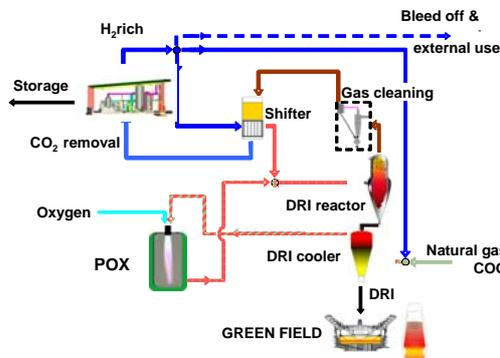
Figure 1. Schematic Layout of the ULCORED concept
