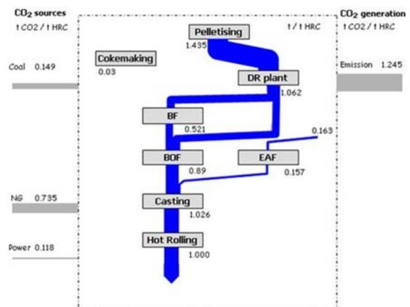
Figure 2. Detailed flowsheet for optimised combined use of DRI+LRI in BF and BOF. The BF/BOF route is operated without scrap (i.e. scrap is melted outside the route)
