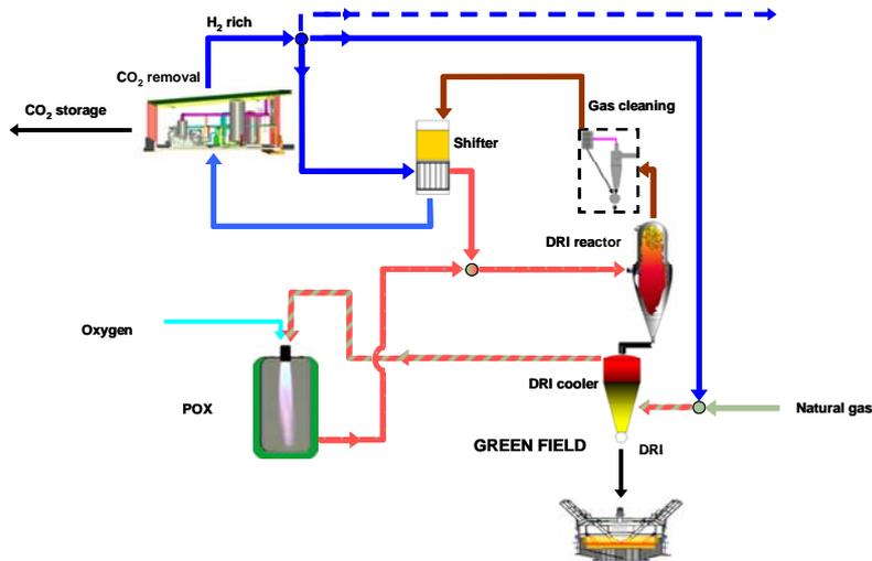
Figure 1. Flow sheet of ULCORED with natural gas
