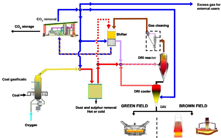
Figure 2. ULCORED with syngas from coal
