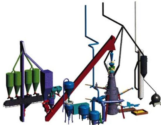
**Figure 2.** Schematic diagram of the LKAB's Experimental Blast Furnace
