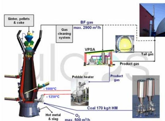
**Figure 4. ULCOS blast furnace at LKAB's EBF plant**
