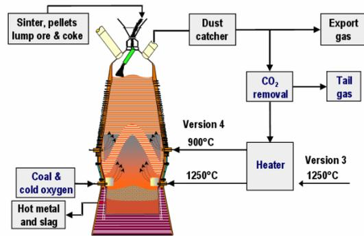
**Figure 3. Process flow of the two versions of the TGRBF**
