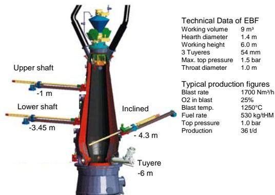
**Figure 1.** The experimental blast furnace
