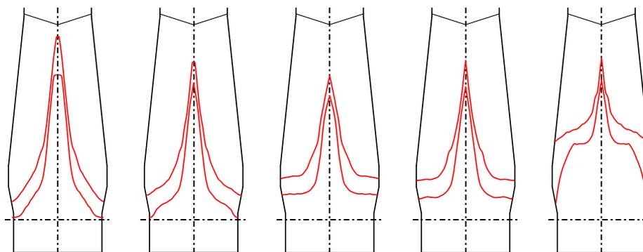
Figure 2. Calculated shape of the cohesive zone (Oct. 96, May 98, Oct. 00, June 01, July 01)
