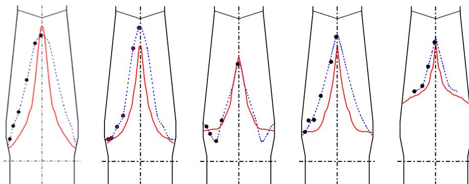
Figure 3. Measured and calculated upper face of the cohesive zone (Oct. 96, May 98, Oct. 00, June 01, July 01)
