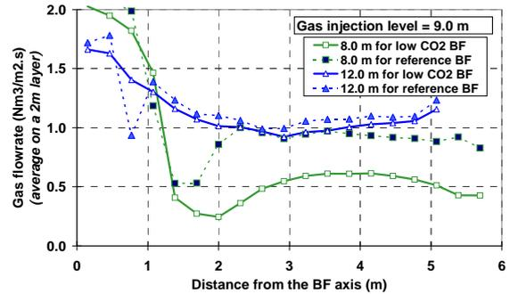
**Figure 5.** Horizontal profiles of gas flow rates for the conventional BF and the ULCOS BF process
