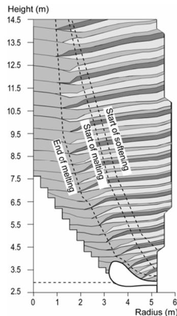
Figure 1. Structure of the cohesive zone calculated by MOGADOR (example)
