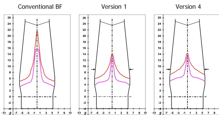
Figure 8. Calculated cohesive zone for versions 1 and 4 of the ULCOS BF compared to conventional BF
