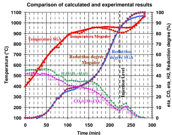
**Figure 7.** Comparison of calculated and experimental progress of reduction degree for the ULCOS BF process
