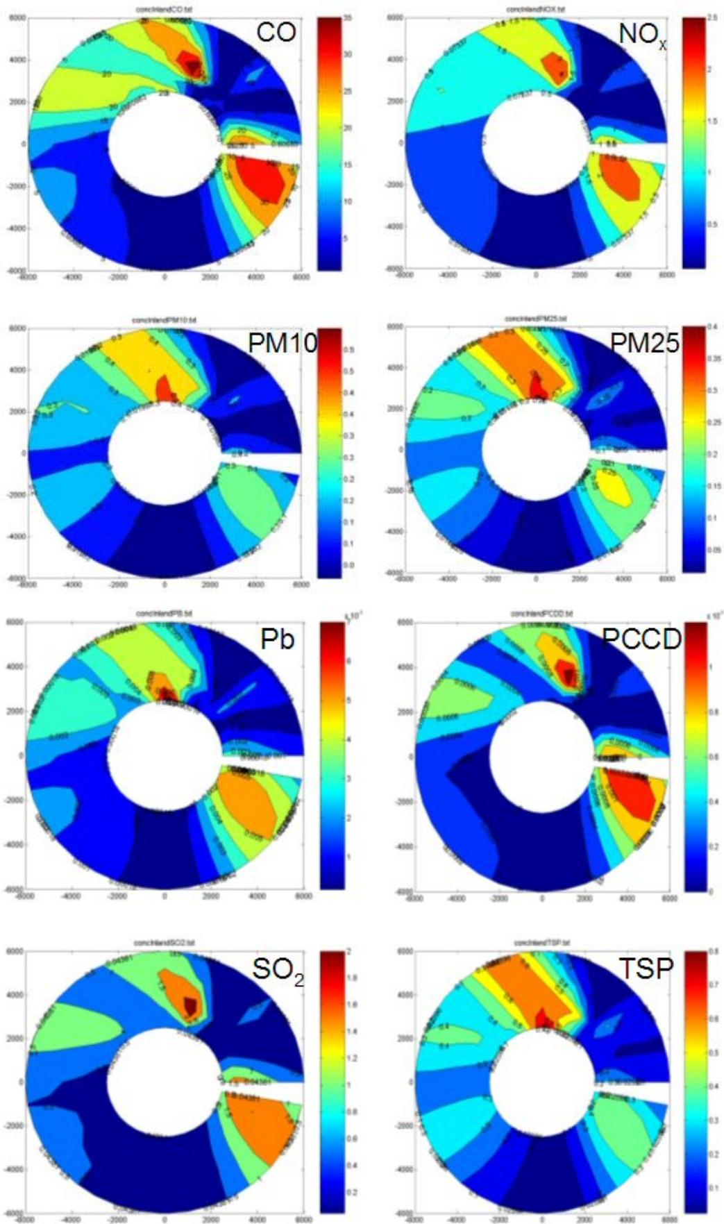
**Figure 4a-h.** The pictures show the results of the AERMOD simulation of air dispersion for the following pollutants (from left top to right bottom): CO, NO<sub>x</sub>, PM<sub>10</sub>, PM<sub>25</sub>, Pb, PCCD, SO<sub>2</sub>, TSP.
