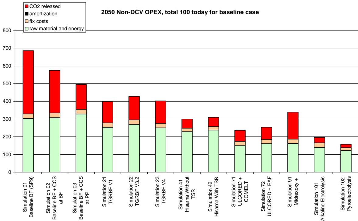
Figure 11 - OPEX for 2050 Non-DCV, Factor2 Europe scenario, index base 100 for today's blast furnace
