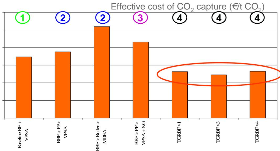
Figure 14 – Cost of avoided CO<sub>2</sub> (CAC) for various solution of implementing CCS on a blast furnace (CO<sub>2</sub> abatement cost figures have been hidden)
