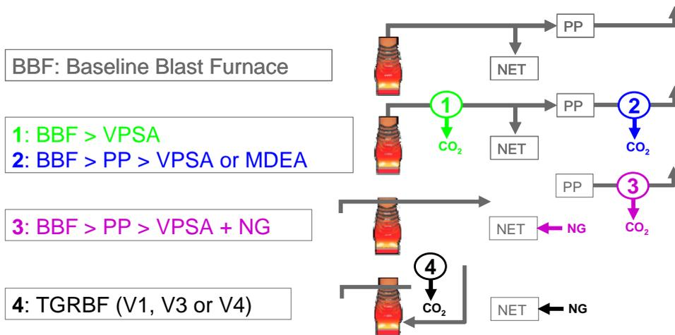
Figure 12 - Various solutions of implementing CCS on a blast furnace
