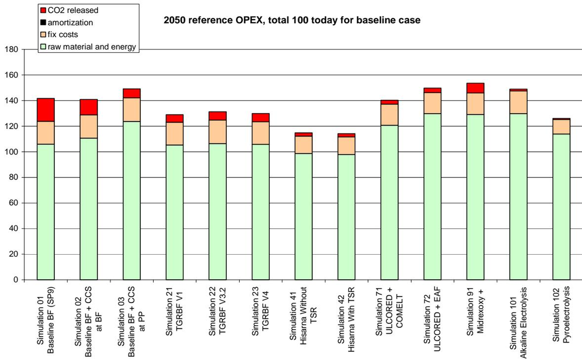
Figure 10 - OPEX for 2050 reference, index base 100 for today's blast furnace
