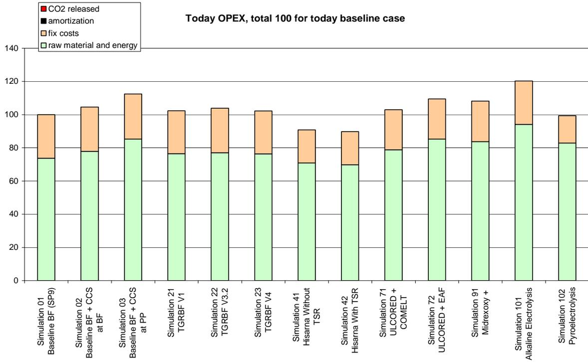
Figure 9 - OPEX today, index base 100 for today's blast furnace
