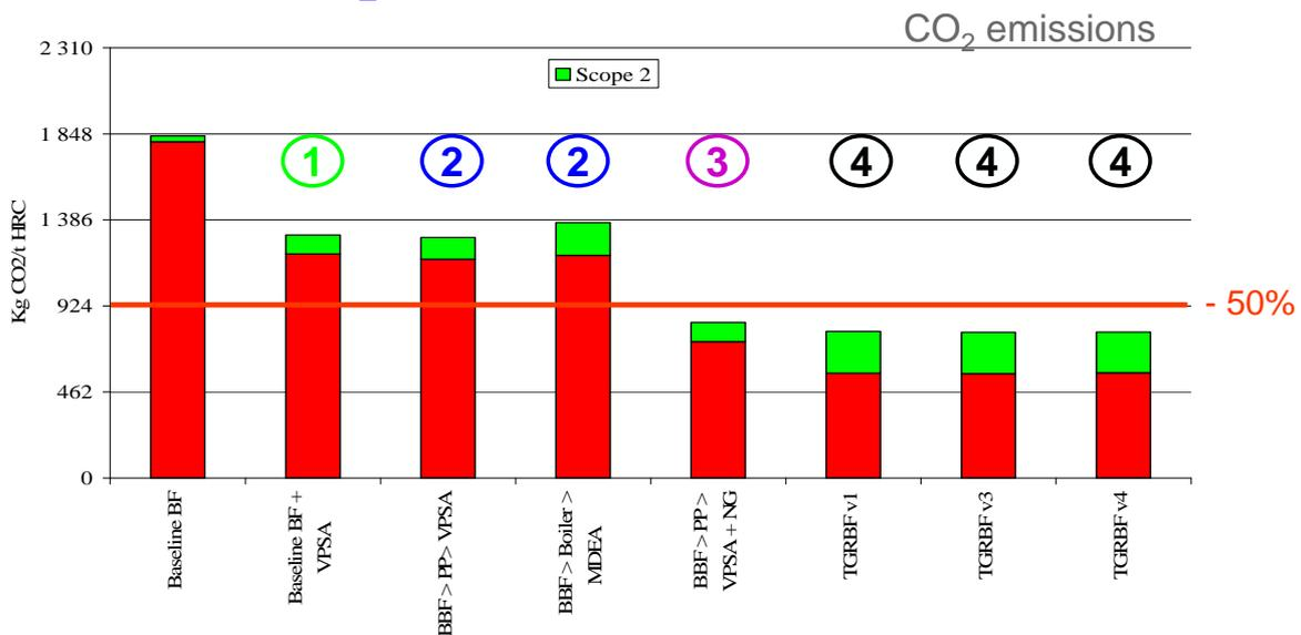
Figure 13 - CO<sub>2</sub> mitigation level for various solution of implementing CCS on a blast furnace (scope I and II CO<sub>2</sub> balances)
