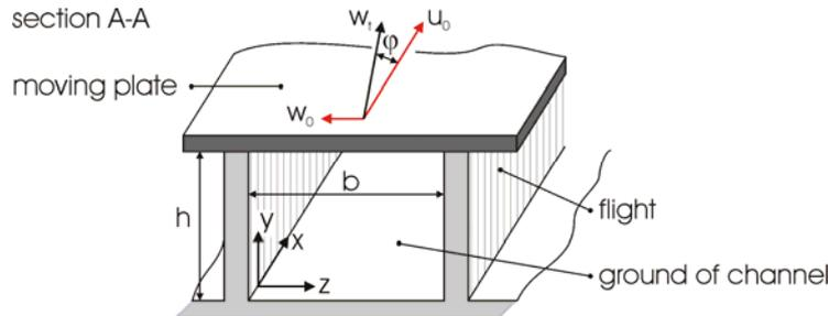
**FIGURE 2:** Planar channel dimensions and channel-fixed velocities.
