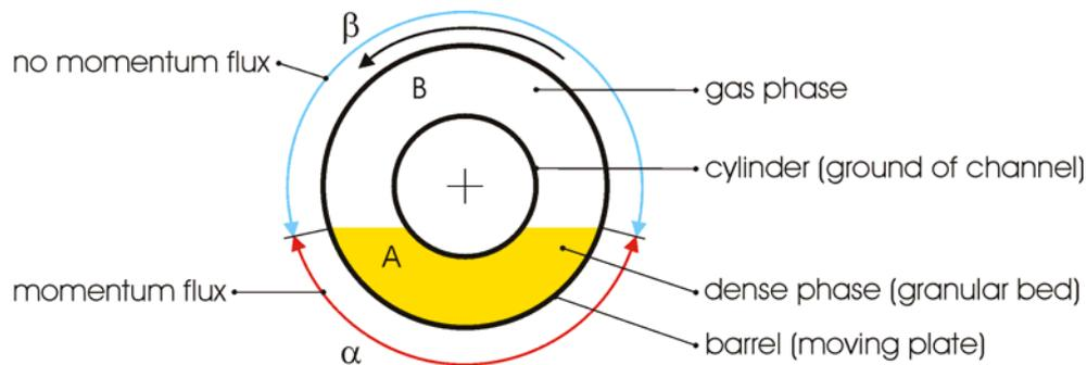
**FIGURE 3:** Partitioning of the phase interfaces
