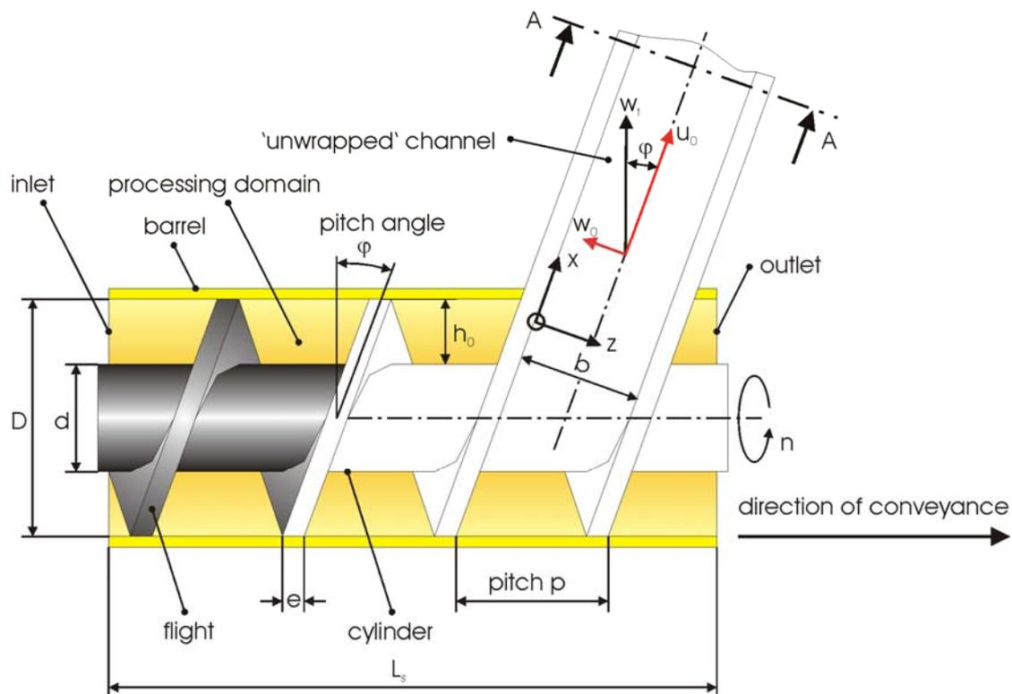
**FIGURE 1:** Transformation of the helical channel into a planar channel
