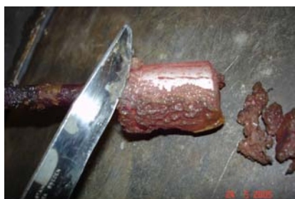
Figure 2. Scraping off the cathode deposit
