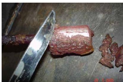
Figure 2. Scraping off the cathode deposit
