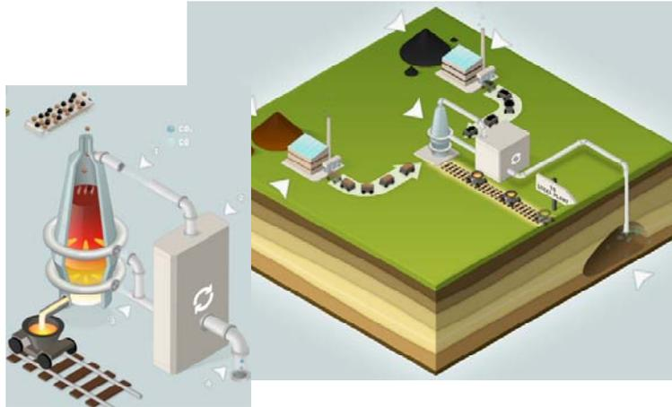
**Figure 4:** Schematics of the TGR-BF process
