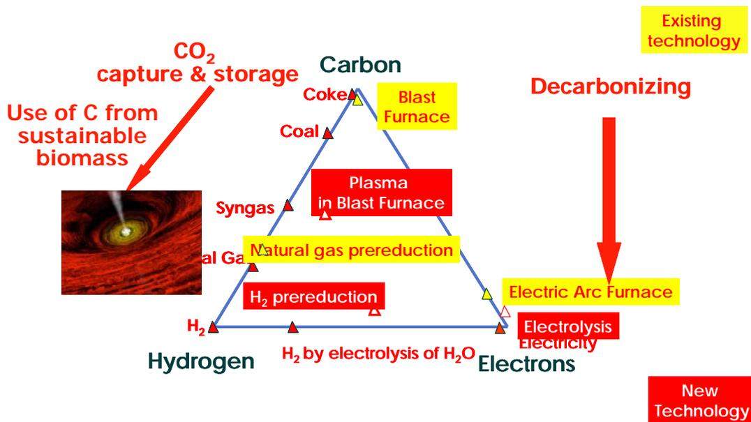
**Figure 3:** pathways to breakthrough technologies for cutting CO<sub>2</sub> emissions from the ore-based steel production routes
