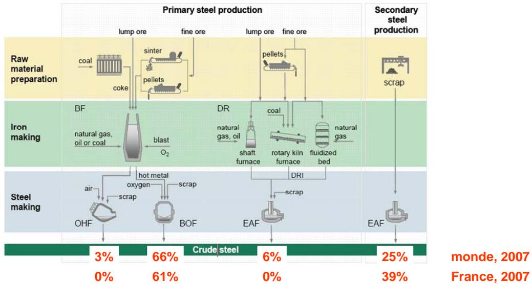
**Figure 1:** Production routes to make steel today, with production shares in the world and in France (BF: Blast Furnace; OHF: Open Hearth Furnace; BOF: Basic Oxygen Furnace; EAF: Electric Arc Furnace; DR: Direct Reduction)
