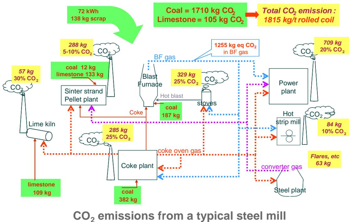
**Figure 2:** Simplified flow sheet of an Integrated Steel Mill, showing carbon-bearing material input (green boxes, highlighted), CO<sub>2</sub> emissions, expressed in volume (kg/t of hot rolled coil) and concentration in the flue gas (volume %).
